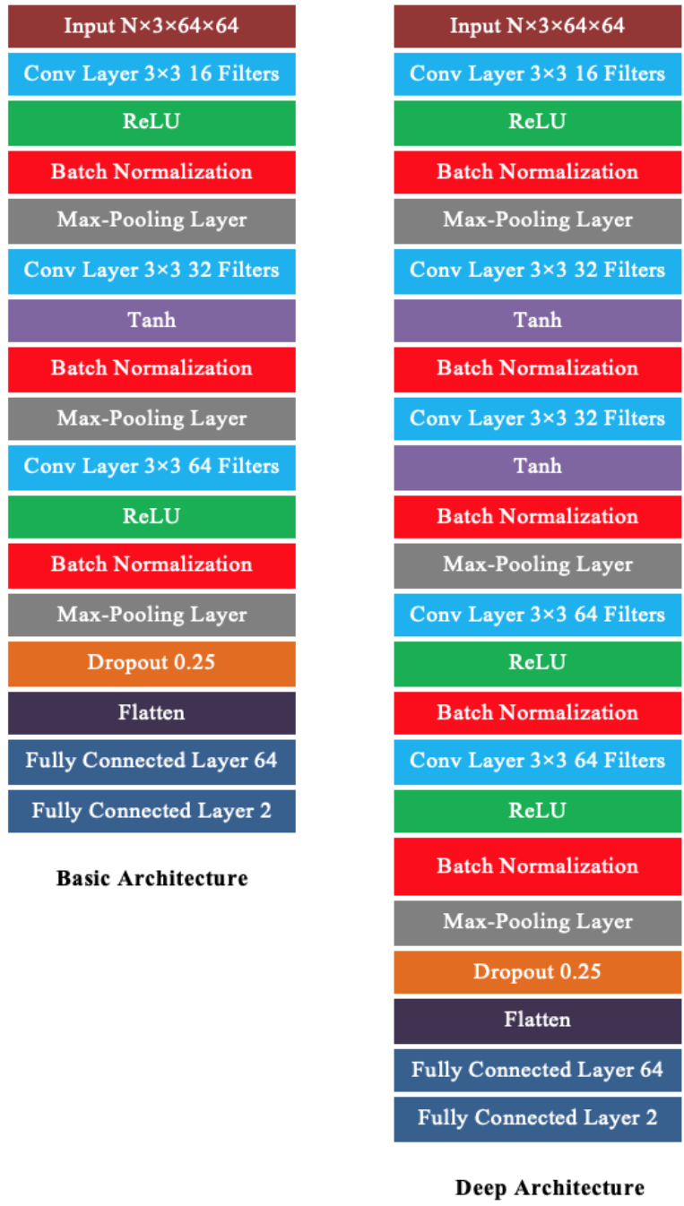
Figure 6. Architectures of Distracted Pedestrians Detector
