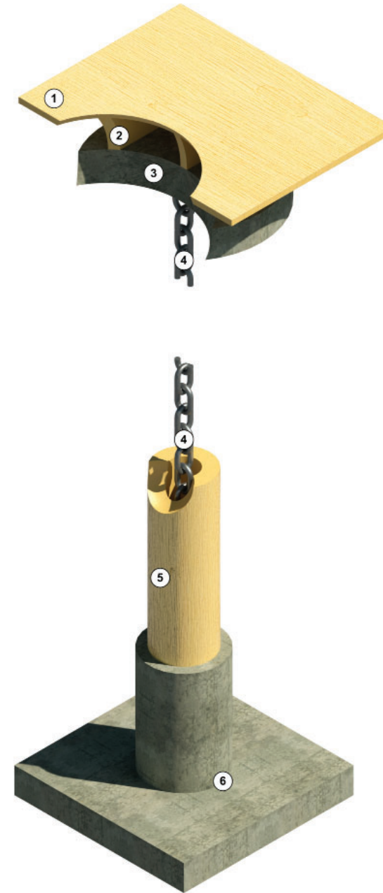
PIER DESIGN LEGEND 1. Wooden Deck 2. Deck Joist 3. Concrete Anchor Pads 4. Iron Retracting Chains 5. Hollow Wooden Pier 6. Concrete Footing
