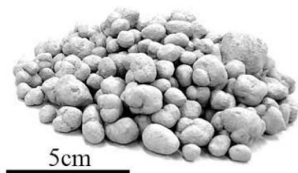
Figure 6. Pelletized lightweight aggregate product. Reprinted from Waste Management, Vol. 29, Gunning et al. [105], 2722-2728, Copyright 2009, with permission from Elsevier.
