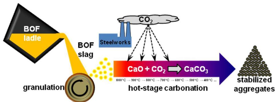
**Figure 3.** Stabilization of basic oxygen furnace slag by hot-stage carbonation treatment. Reprinted from Chemical Engineering Journal, Vol. 203, Santos *et al.* [40], 239-250, Copyright 2012, with permission from Elsevier.
