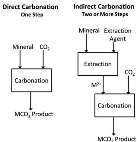
**Figure 1.** Direct (one step) mineral carbonation (left), and indirect (two or more steps) mineral carbonation (right); M refers to either calcium or magnesium. Reprinted from Progress in Energy and Combustion Science, Vol. 38, Bobicki *et al.* [24], 302-320, Copyright 2011, with permission from Elsevier.
