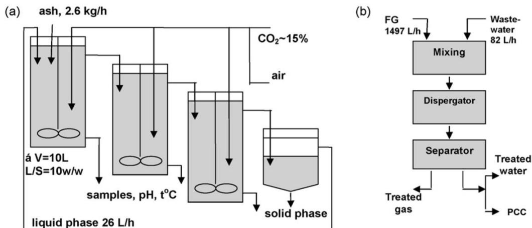
**Figure 5.** Experimental cascading reactors for carbonation of oil-shale ash suspension (a) and alkaline wastewater (b). Reprinted from Journal of Hazardous Materials, Vol. 174, Uibu *et al.* [98], 209-214, Copyright 2009, with permission from Elsevier.
